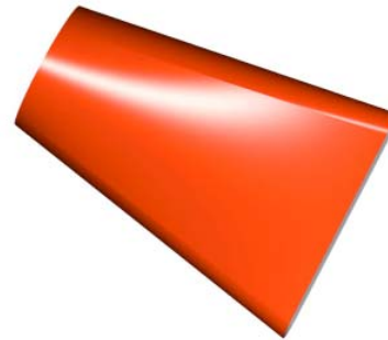
Tangent discontinuity up to 12.0 degrees with uniform parameterization
